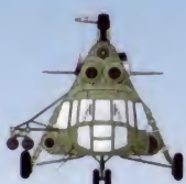
Mi-8 'HIP-C': With two engines and five main rotor blades, the Mi-8 'Hip-C' became the main assault helicopter of the USSR.
